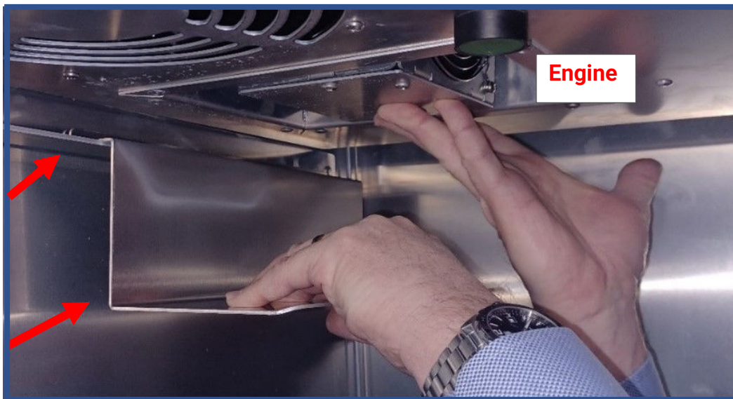
Operator lifting Engine to slide Shelf onto the ledge
